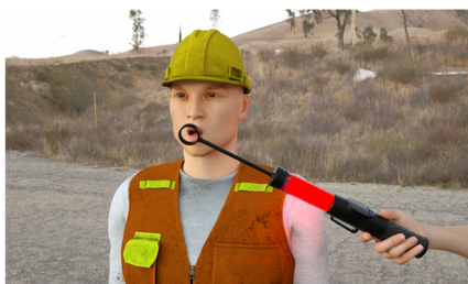
Extended mouthpiece to prevent blowing directly to the operator
