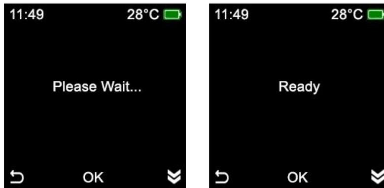
6. Insert a mouthpiece, take a deep breath and blow CONTINUOUSLY until a click sound is heard. A beeping tone will be heard when blowing. Test result will display on the LCD.
